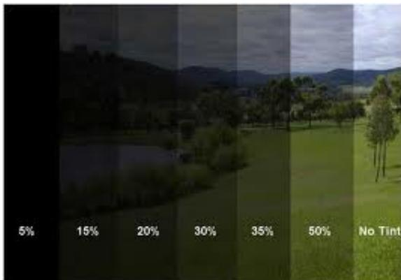
**Tinted glass**, however, provides an easy solution to these problems. It has become the most popular use of tinted glass is in windows of homes and commercial buildings. It refers to any glass that has been treated with a material such as a film that reduces the transmission of light through it. Glass can be tinted with various types of film, which block and/or reflect different amounts and types of light, according to the needs and preferences of the consumer.
